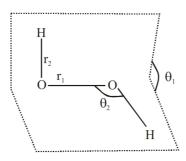
$r_1 = 98.5 \text{ pm}, r_2 = 145.8 \text{ pm}, \ \theta_1 = 90.2^0, \ \theta_2 = 101.9^0 \text{ (Crystalline phase)}$
